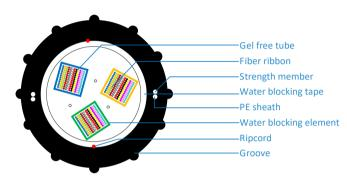
Note: The quantity, specifications and positions of the strength members may vary depending on the installation conditions.
