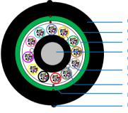
Outer sheath Corrugated steel tape Water blocking tape Central strength member (FRP, PE coated if necessary) Loose tube, fibers and water blocking yarns Water blocking yarns Ripcord Ripcord identifier
